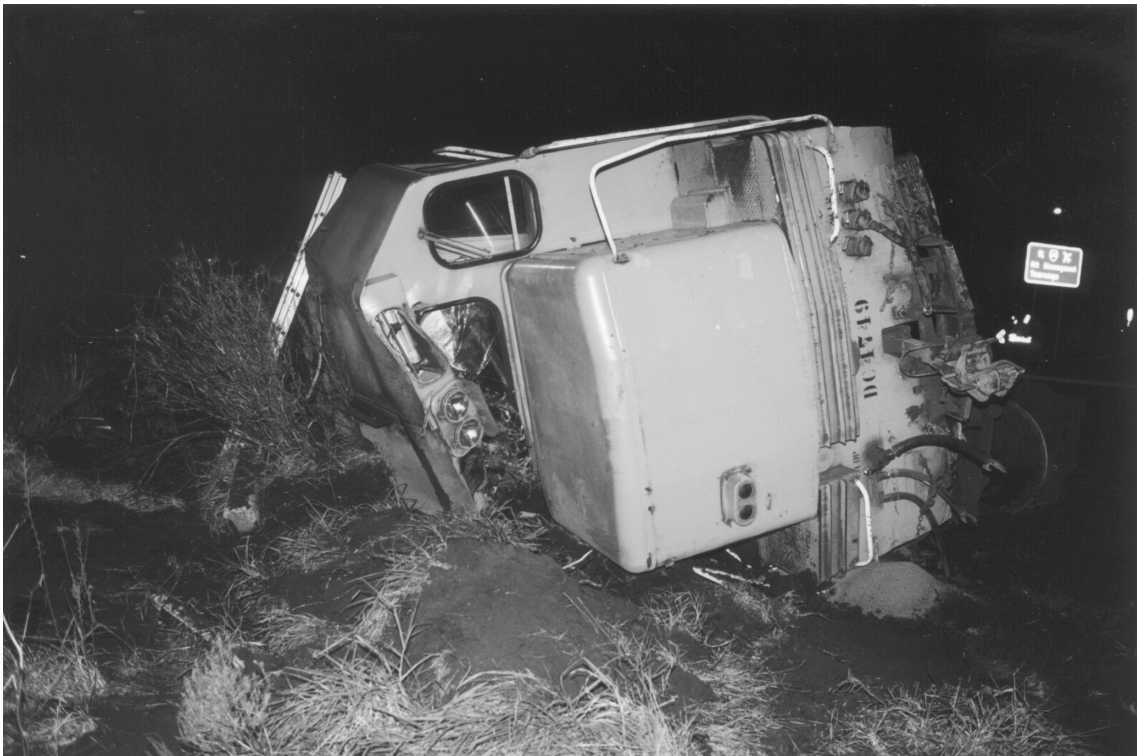
Figure 3 The leading (cab) end of DC 4749 looking in direction of travel (the locomotive had pivoted end to end before coming to rest)
